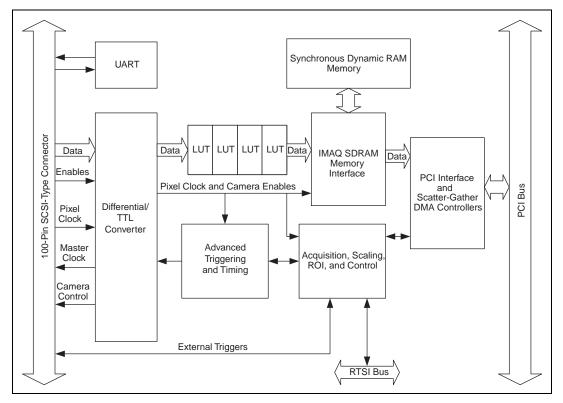
Figure 3-1. PCI-1424 Block Diagram
