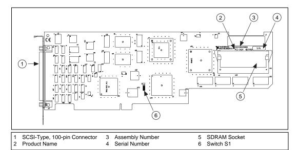
Figure 2-2. PCI-1424 Parts Locator Diagram
